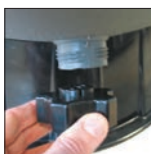
Sand easily accessible by removing the collar
